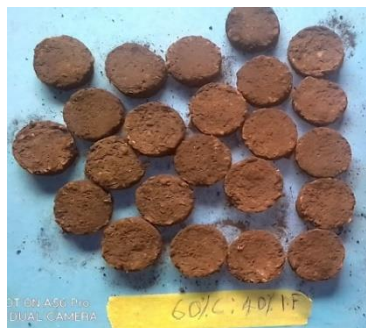
Figure 1b: 60% coal: 40% iron filings pellets
